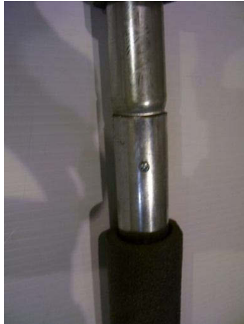
Upper (dog leg) and Straight Sections of Upright Posts joined and secured with a Screw.
